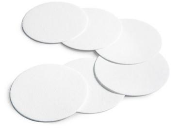
Grade 470 papers are made of cellulose and diatomaceous earth and offer a much better separating capability than pure cellulose papers at the same rate of filtration. This grade quickly retains the finest particles at high flow rates.
