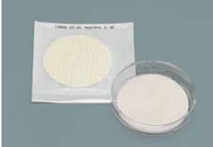
Nutrient pad set with membrane filter
