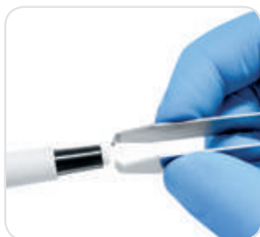
Safe-Cone Filters protect the pipette from contamination, and should be changed regularly.
