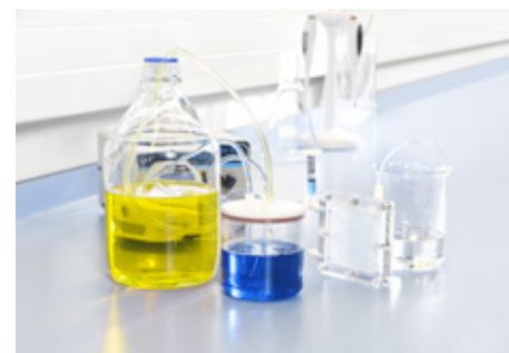
Figure 2: Diafiltration system set up for buffer exchange. Culture medium concentrate can be seen in the center of the image. 1 L 25 mM sodium acetate (exchange buffer) can be seen connected to the system on the left of the image.
