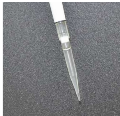
Figure 1. Pipetting BSA solution (1 mg/ml) with slow speed (Picus® setting 1)
