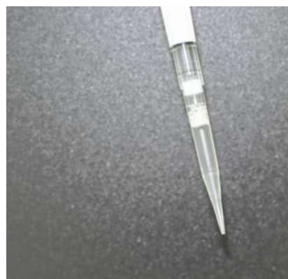
Figure 2. Pipetting BSA solution (1 mg/ml) with fast speed (Picus® setting 9).
